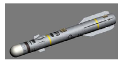
Properties: Flight Profile - Terrain Following, Bearing-Only Launch (BOL), Flight Profile - Level Cruise Flight Targets: Surface Vessel, Mobile Target - Soft, Mobile Target - Hardened
