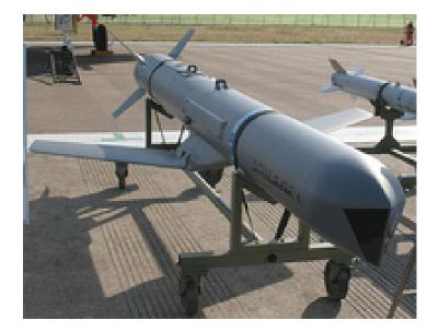
$Properties: Flight\ Profile\ -\ Terrain\ Following,\ We apon\ -\ INS\ w/\ GNSS\ Navigation,\ Terminal\ Maneuver\ -\ Pop-Up,$
