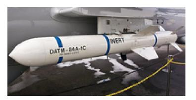
Properties: Home On Jam (HOJ), Flight Profile - Terrain Following, Search Pattern, Bearing-Only Launch (BOL),
