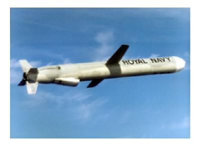
Properties: Flight Profile - Terrain Following, Weapon - INS w/ GNSS Navigation, Weapon - Pre-Briefed Target Only,
