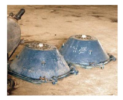
Properties: Mine - Magnetic Fuze, Total-Field Magnetometer, Mine - Passive Acoustic Fuze, Broad-Band (Simple), Mine - Delay Counter, Mine - Arming Delay Targets: Surface Vessel, Submarine
