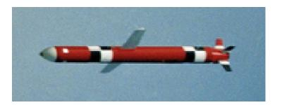
Properties: Flight Profile - Terrain Following, Weapon - INS w/ GNSS Navigation, Weapon - Pre-Briefed Target Only,
