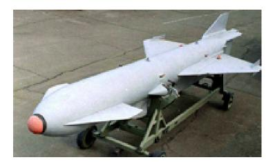
Properties: Flight Profile - Terrain Following, Bearing-Only Launch (BOL), Weapon - INS Navigation, Flight Profile -
