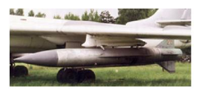
Properties: Home On Jam (HOJ), Bearing-Only Launch (BOL), Weapon - INS Navigation, Level Cruise Flight Targets: Surface Vessel
