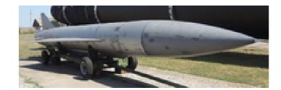
Properties: Home On Jam (HOJ), Bearing-Only Launch (BOL), Weapon - INS Navigation, Flight Profile - Level Cruise Flight Targets: Surface Vessel
