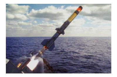
Properties: Bearing-Only Launch (BOL), Weapon - INS Navigation, Flight Profile - Level Cruise Flight
