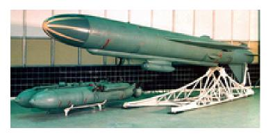
Properties: Home On Jam (HOJ), Flight Profile - Terrain Following, Search Pattern, Bearing-Only Launch (BOL),
