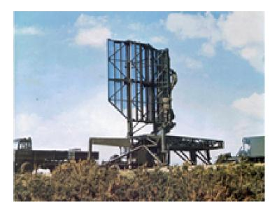
Sensors / EW: - AR-3D - Radar, Radar, Air Search, 3D Long-Range, Max range: 555.6 km
