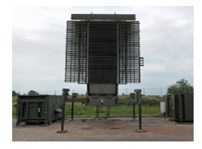
Sensors / EW: - RAT-31DL - Radar, Radar, Air Search, 3D Long-Range, Max range: 444.5 km
