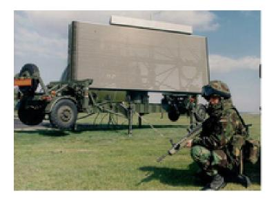
Sensors / EW: - Type 101 [AR-327] - (1998) Radar, Radar, Air Search, 3D Long-Range, Max range: 555.6 km
