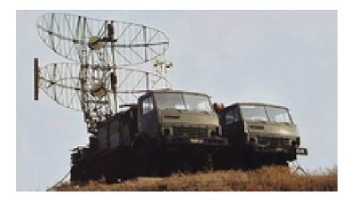
Sensors / EW: - Flat Face E [P-19, Kasta 2E Upgrade] - (1RL134, Danube) Radar, Radar, Air Search, 2D Medium-Range, Max range: 250 km
