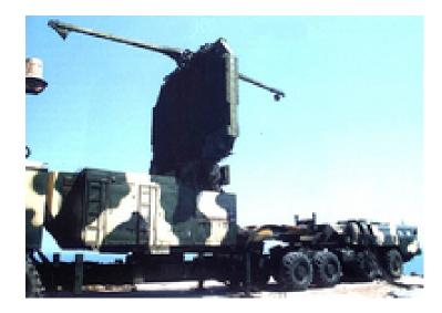
Sensors / EW: - Big Bird C [64N6] - (SA-20) Radar, Radar, Air Search, 3D Long-Range, Max range: 601.9 km
