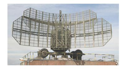
Sensors / EW: - Bar Lock B [P-37] - Radar, Radar, Air Search, 3D Long-Range, Max range: 463 km
