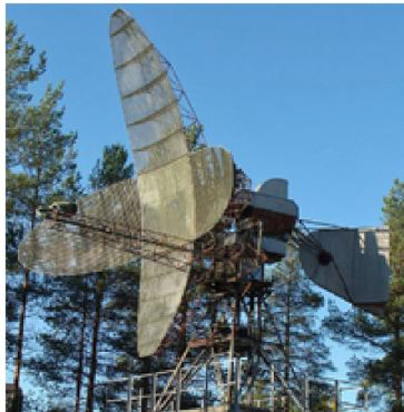
Sensors / EW: - VRRVY - (Finland) Radar, Radar, Air & Surface Search, 3D Medium-Range, Max range: 277.8 km
