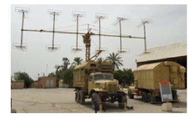
Sensors / EW: - Spoon Rest C [P-12] - Radar, Radar, Air Search, 2D Medium-Range, Max range: 277.8 km
