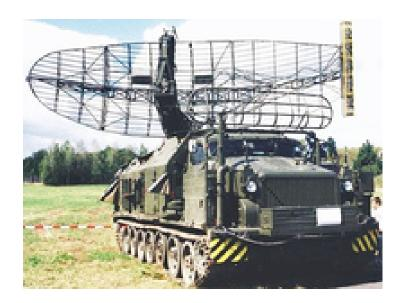
Sensors / EW: - Long Track [P-40] - (1S12) Radar, Radar, Air Search, 3D Long-Range, Max range: 370.4 km
