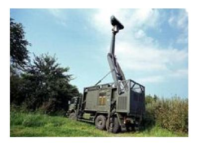
Sensors / EW: - Giraffe AMB 3D - (2001) Radar, Radar, Target Indicator, 3D Surface-to-Air, Max range: 148.2 km
