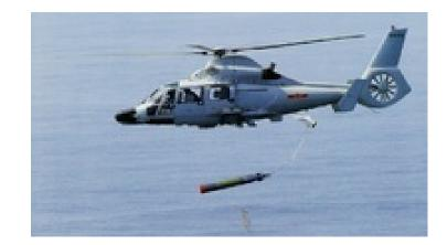
Sensors / EW: - China Type 605 - Dipping Sonar, Active-Only, Dipping Sonar, Active-Only Search & Track, Max range: 5.6 km
