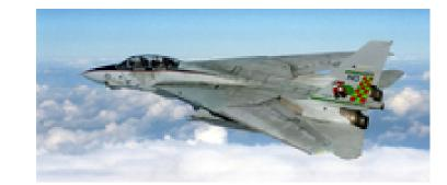
Sensors / EW: - AN/AAS-42 - Infrared, IRST, Imaging Infrared Search and Track, Max range: 185.2 km - AN/ALQ-165 ASPJ - ECM, DECM, Defensive ECM, Max range: 0 km
