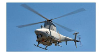
Sensors / EW: - AN/ZPY-4(V)1 [RDR-1700B+] - Radar, Radar, Surface Search, Medium-Range, Max range: 148.2 km - AN/AAQ-22 BRITE Star II [IR] - (Group, Rangefinder) Infrared, Infrared, Target Search, Tracking and Identification Camera, Max range: 111.1 km
