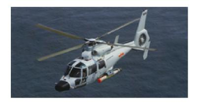
Sensors / EW: - AN/AQS-13B - Dipping Sonar, Active-Only, Dipping Sonar, Active-Only Search & Track, Max range: 5.6 km
