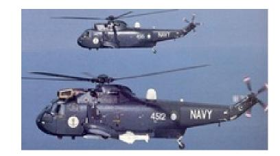
Sensors / EW: - ARI.5955 - (AWS.391) Radar, Radar, Surface Search, Short-Range, Max range: 92.6 km - Type 195 - (1967) Dipping Sonar, Active/Passive, Dipping Sonar, Active/Passive Search & Track, Max range: 5.6 km
