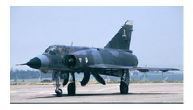
Sensors / EW: - Cyrano II bis - Radar, Radar, FCR, Air-to-Air & Air-to-Surface, Short-Range, Max range: 50 km - BU/BZ - ESM, RWR, Radar Warning Receiver, Max range: 222.2 km
