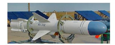
Properties: Home On Jam (HOJ), Flight Profile - Terrain Following, Search Pattern, Bearing-Only Launch (BOL), Weapon - INS Navigation, Terminal Maneuver - Pop-Up, Flight Profile - Level Cruise Flight Targets: Surface Vessel
