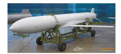
Properties: Flight Profile - Terrain Following, Weapon - TERCOM Navigation, Weapon - Pre-Briefed Target Only, Flight Profile - Level Cruise Flight Targets: Land Structure - Soft, Land Structure - Hardened, Runway
