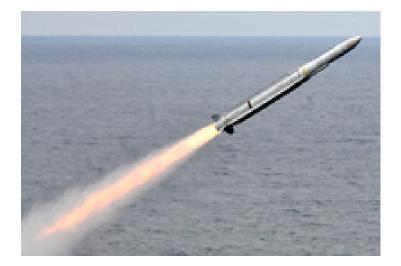
Properties: Illuminate at Launch, Anti-Air All-Aspect, Capable vs Seaskimmer, Flight Profile - Level Cruise Flight Targets: Aircraft, Helicopter, Missile, Surface Vessel
