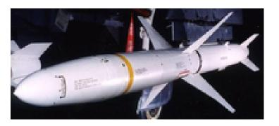
Properties: Home On Jam (HOJ), ARM Target Memory, Bearing-Only Launch (BOL), Flight Profile - Level Cruise
