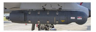
Properties: Pod - Night Navigation/Attack (Incl. Bomb, Rocket Delivery)
