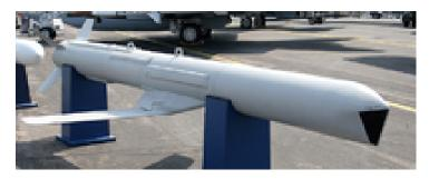
Properties: Flight Profile - Terrain Following, Weapon - INS w/ GNSS Navigation, Terminal Maneuver - Pop-Up,
