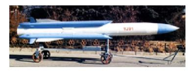
Properties: Home On Jam (HOJ), Flight Profile - Terrain Following, Bearing-Only Launch (BOL), Weapon - INS
