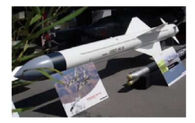
Properties: Home On Jam (HOJ), Flight Profile - Terrain Following, Search Pattern, Bearing-Only Launch (BOL), Weapon - INS Navigation, Terminal Maneuver - Pop-Up, Flight Profile - Level Cruise Flight Targets: Surface Vessel
