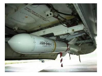
Properties: Home On Jam (HOJ), Flight Profile - Terrain Following, Search Pattern, Bearing-Only Launch (BOL),
