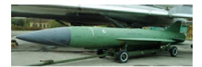
Properties: Home On Jam (HOJ), Bearing-Only Launch (BOL), Weapon - INS Navigation, Flight Profile - Level Cruise Flight Targets: Surface Vessel
