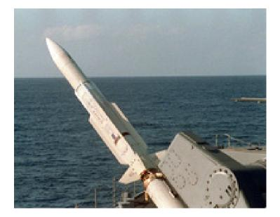
Properties: Terminal Illumination, Home On Jam (HOJ), Anti-Air All-Aspect, Multi-Stage Missile, Flight Profile -
