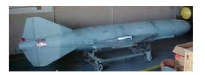
Properties: Home On Jam (HOJ), Flight Profile - Terrain Following, Bearing-Only Launch (BOL), Weapon - INS Navigation, Weapon - Pre-Briefed Target Only, Terminal Maneuver - Pop-Up, Flight Profile - Level Cruise Flight Targets: Surface Vessel, Land Structure - Soft, Land Structure - Hardened
