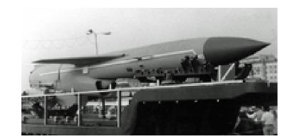
Properties: Home On Jam (HOJ), Search Pattern, Bearing-Only Launch (BOL), Weapon - INS Navigation, Flight Profile - Level Cruise Flight Targets: Surface Vessel
