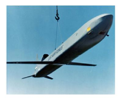
Properties: Flight Profile - Terrain Following, Weapon - TERCOM Navigation, Weapon - Pre-Briefed Target Only, Flight Profile - Level Cruise Flight Targets: Land Structure - Soft, Land Structure - Hardened, Runway
