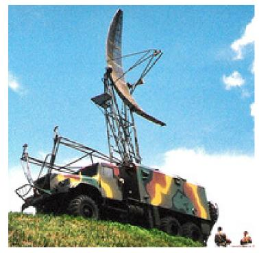
Sensors / EW: - Thin Skin B HF [PRV-16] - Radar, Radar, Height-Finder, Long-Range, Max range: 296.3 km
