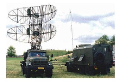
Sensors / EW: - Squat Eye [P-15M(2)] - Radar, Radar, Air Search, 2D Medium-Range, Max range: 203.7 km
