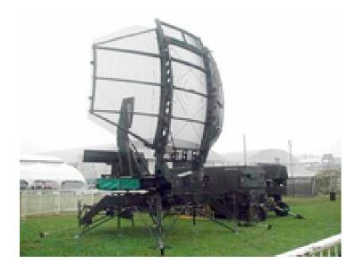
Sensors / EW: - AN/TPS-73 - Radar, Radar, Air Search, 2D Medium-Range, Max range: 148.2 km
