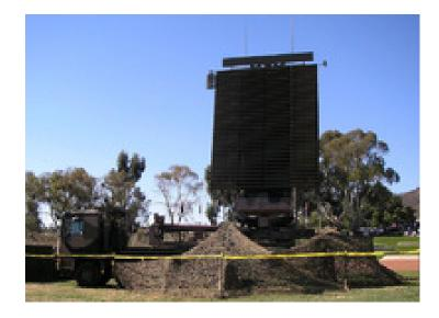
Sensors / EW: - AN/TPS-77 - (AN/FPS-117) Radar, Radar, Air Search, 3D Long-Range, Max range: 555.6 km
