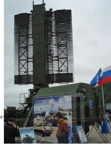
Sensors / EW: - 59N6 Protivnik-GE - Radar, Radar, Air Search, 3D Long-
