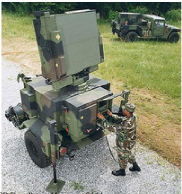
Sensors / EW: - AN/MPQ-64 Sentinel - (1994) Radar, Radar, Air Search, 3D Short-Range, Max range: 74.1 km
