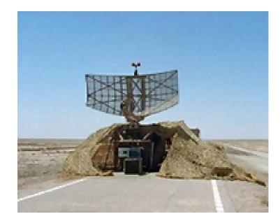
Sensors / EW: - Watchman (T) - Radar, Radar, Air & Surface Search, 2D Medium-Range, Max range: 222.2 km
