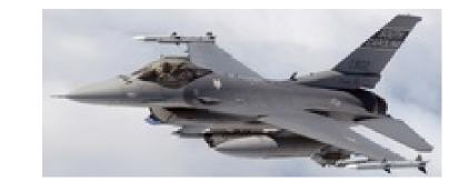
Sensors / EW: - AN/APG-68(V)5 - Radar, Radar, FCR, Air-to-Air & Air-to-Surface, Medium-Range, Max range: 111.1 km
