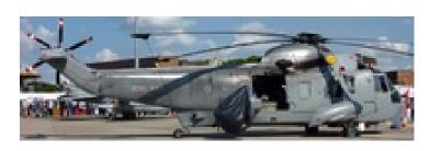
Sensors / EW: - Searchwater 2000 AEW - (Sea King ASaC.7) Radar, Radar, Air & Surface Search, 3D Long-Range, Max range: 370.4 km
